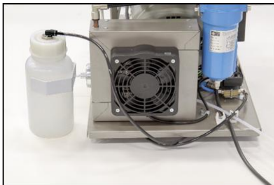
Fig. 7: Connection of condensate collection vessel
