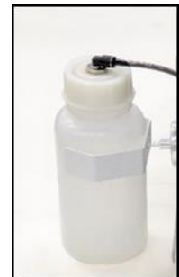
Fig. 11: Check of condensate collection vessel
